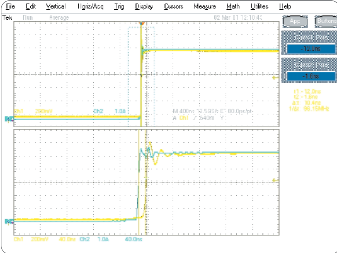
▶ Figure 2. Propagation delay for a voltage and current signal.
