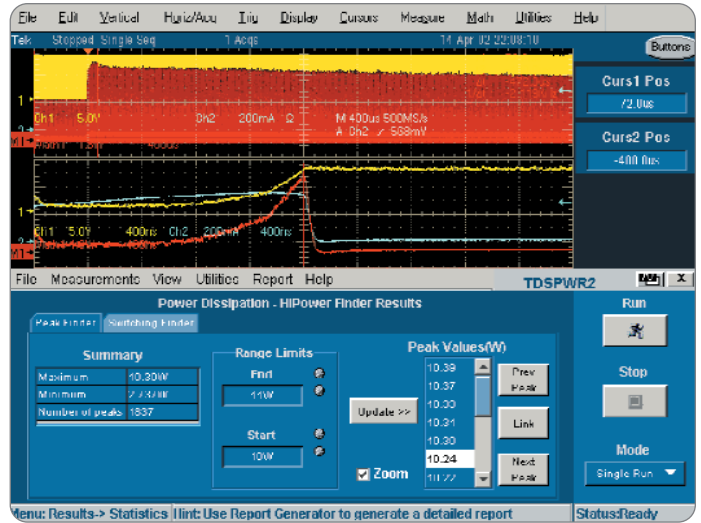
► Figure 7. HiPower Finder and scope zoom can be used for further analysis.
